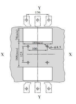
Plug type/Back-plate wiring(3P/4P)
